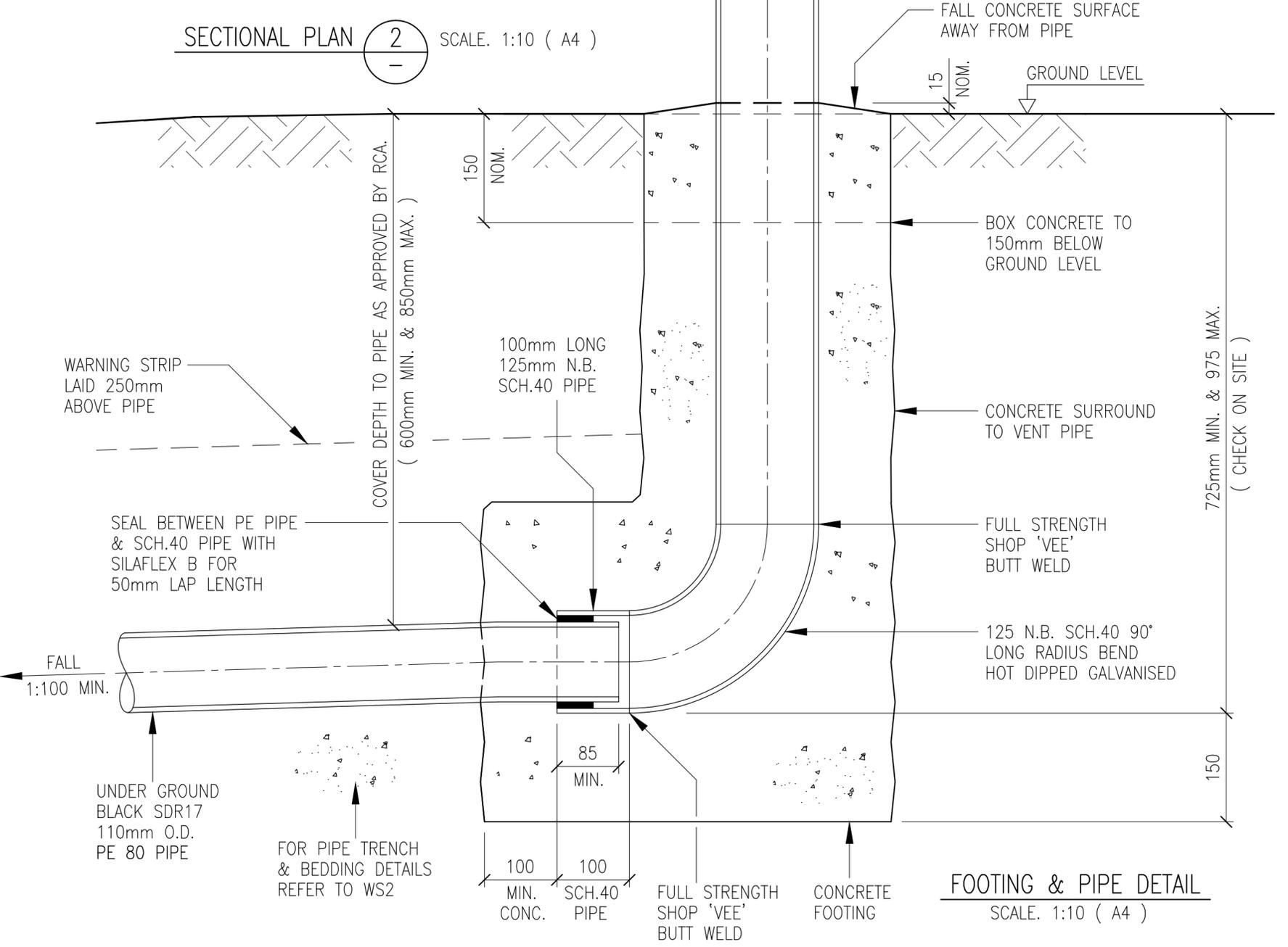
**FOOTING & PIPE DETAIL** SCALE: 1:10 ( A4 )
