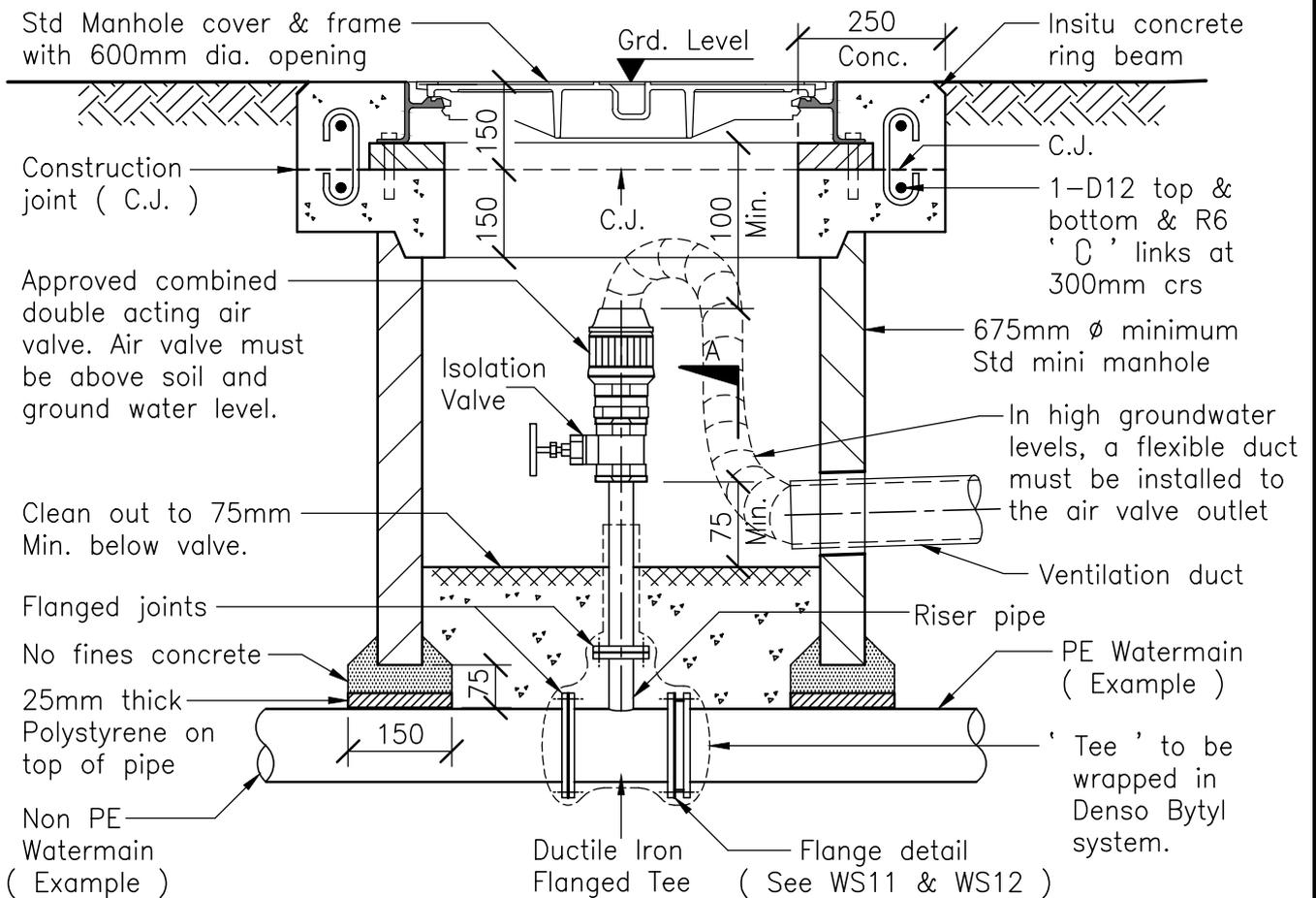
**STANDARD AIR RELEASE VALVE & VALVE CHAMBER DETAIL**
