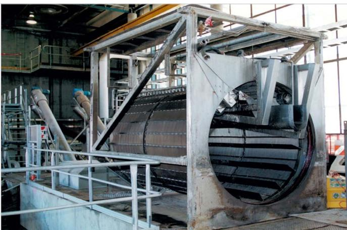
A view of one of the stainless steel fine screens prior to installation.
