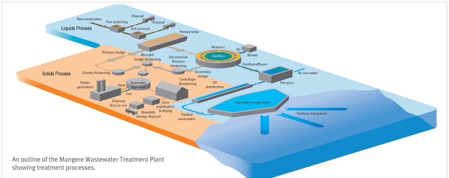
In each unit, eight reactor compartments (four anoxic and four aerobic) are arranged concentrically around an inner clarifier. Effluent from the primary sedimentation tanks is fed proportionately (via the interstage pumping station and splitter boxes) into the anoxic compartments of the reactor.
