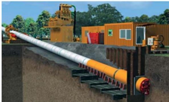
Figure 4-3 Overview of Direct Pipe Installation
