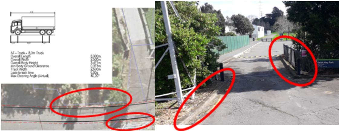
*If we look more closely at the tracking plot, we can see that the tracking in fact illustrates the truck overlapping the side of the bridge structure on one side, and coming close to an electric pylon on the other.*
