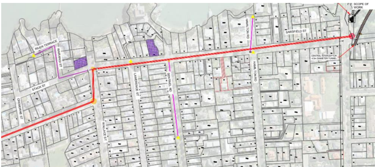
Figure 4-2: Four interception pipelines (shown in pink), along with the EOP connections (yellow triangles) in the eastern portion of the alignment
