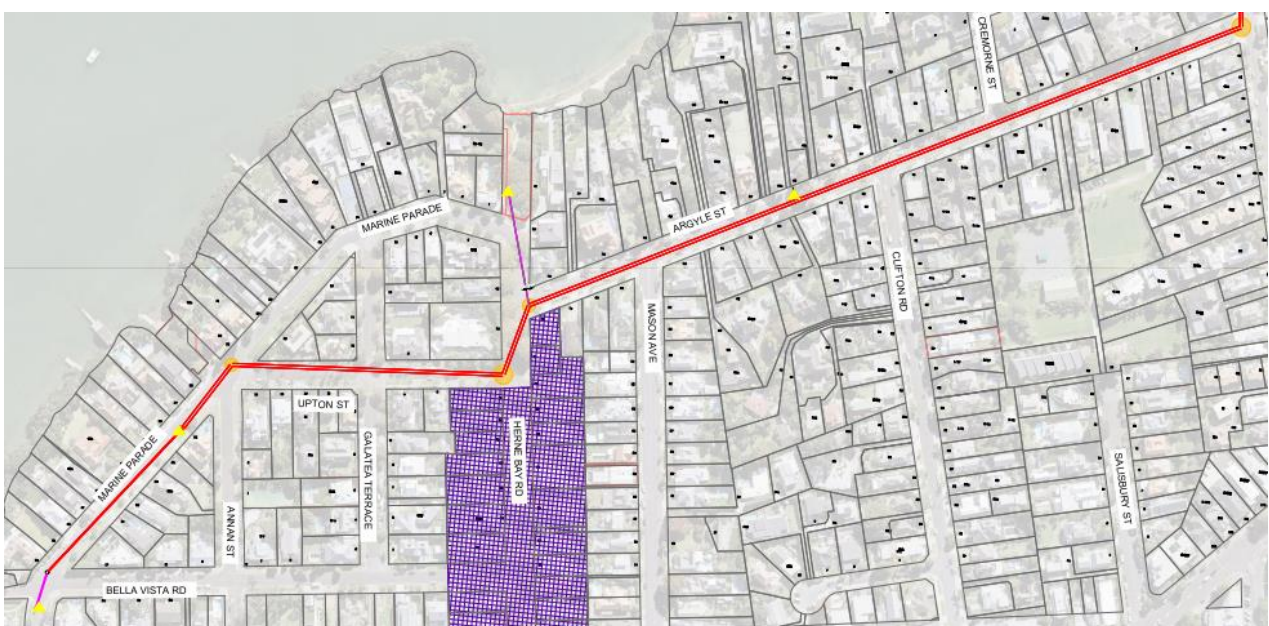
Figure 4-3: Pipe extension from Shaft Eight to EOP 199 (shown in pink), along with the EOP connections (yellow triangles) in the western portion of the alignment
