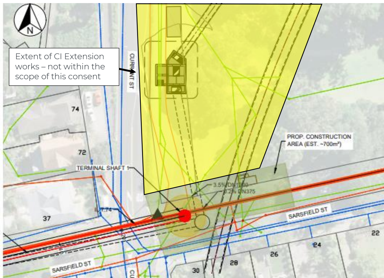
Figure 4-4: Location of Shaft One, with the connection to the CI drop shaft chamber to the north
