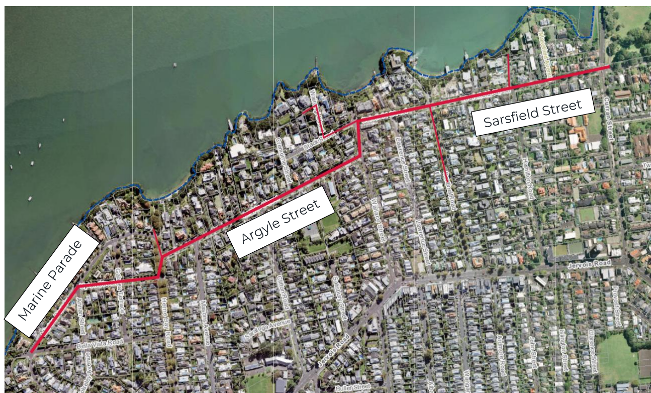
Figure 4-1: Alignment of the tunnel and interception pipelines for the Project
