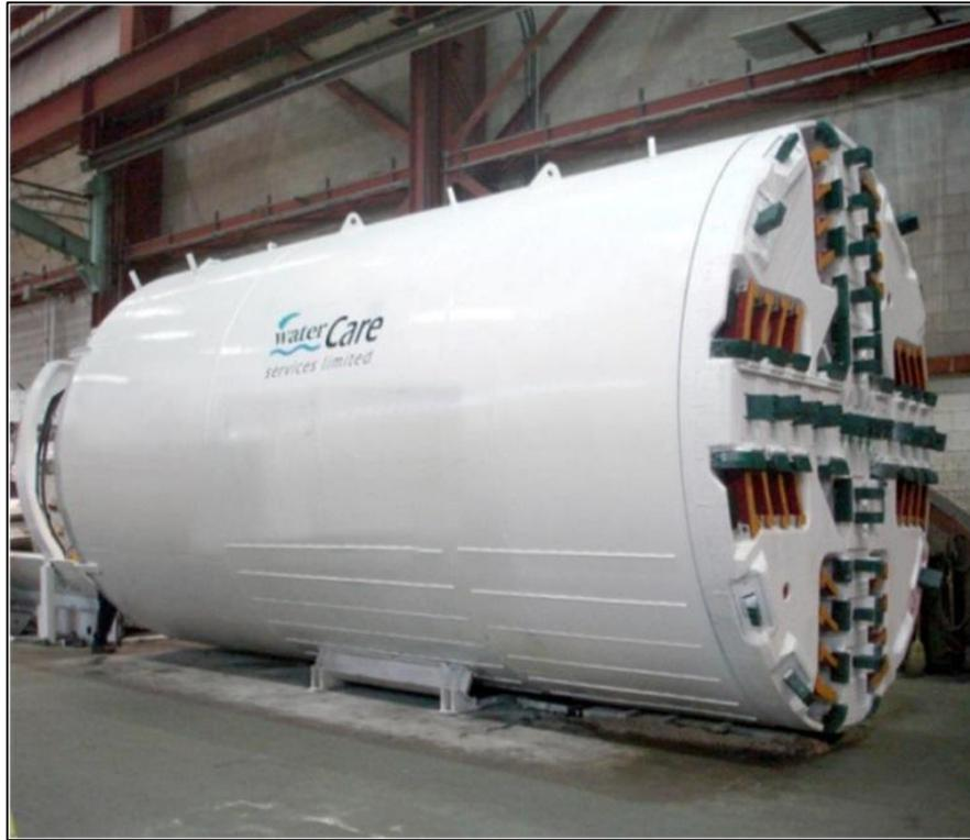
**Figure 3.2 – Example of a TBM**
