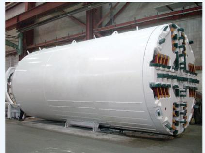
The tunnel boring machine used in the project Hobson Bay tunnel.
