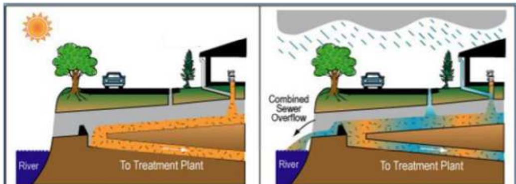
**Figure 2: Operation of typical combined sewer system**
