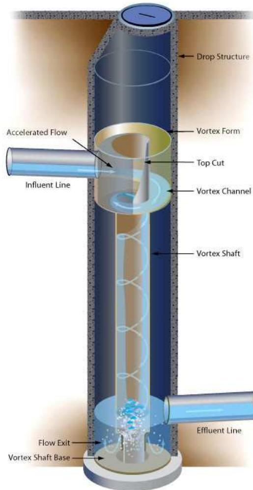
**Figure 4: Typical Vortex Drop Shaft Arrangement (note: the effluent line connects to the main tunnel access shaft)**
