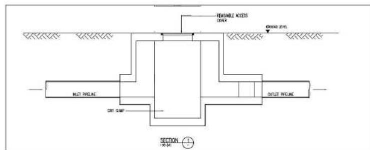
Figure 5-5 Typical grit trap section
