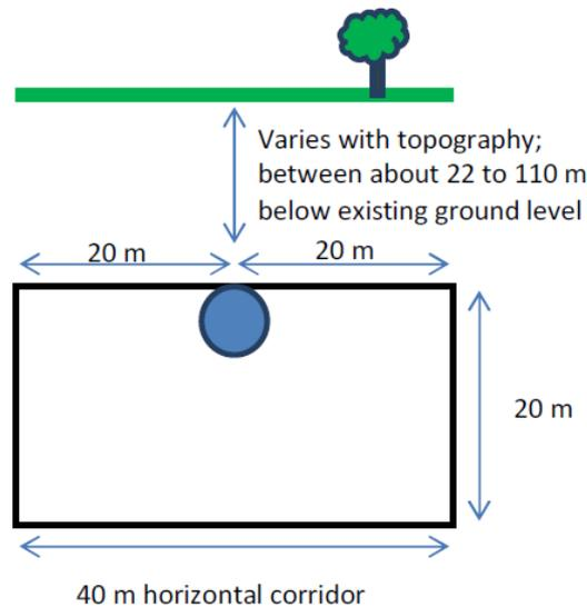
**Figure 2: Main tunnel vertical and horizontal corridor**
