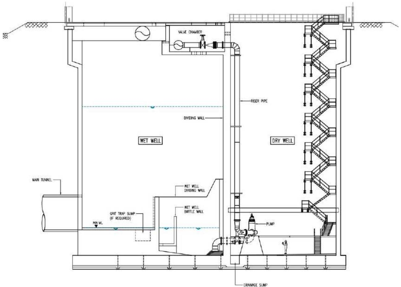
**Figure 6: Pump station wet well/dry well arrangement**
