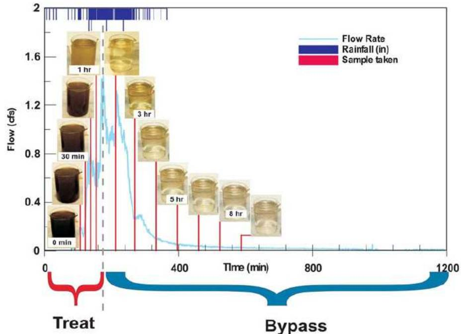
**Figure 1: Stormwater First Flush Contaminant Characterisation**
