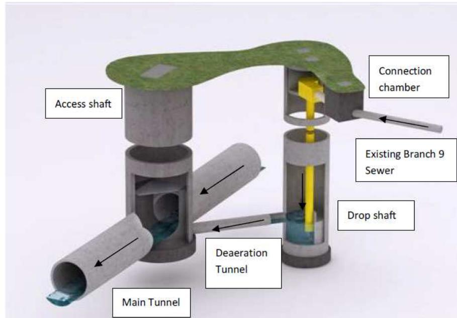
**Figure 3: Indicative arrangement of access shaft, drop shaft, and de-aeration tunnel**
