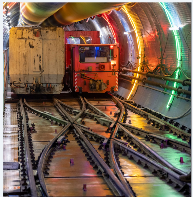
In the main CI tunnel, the electric spoil haulage locomotive is ready for its next trip - Aug 2022
