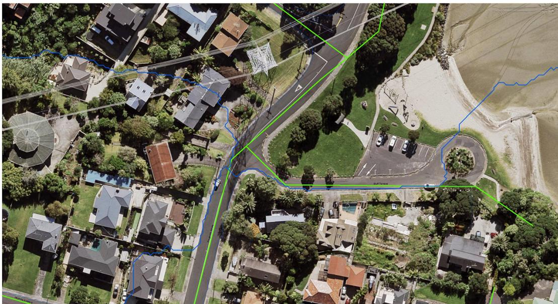
Figure 2 Overland Flow Paths from 2017 LIDAR
