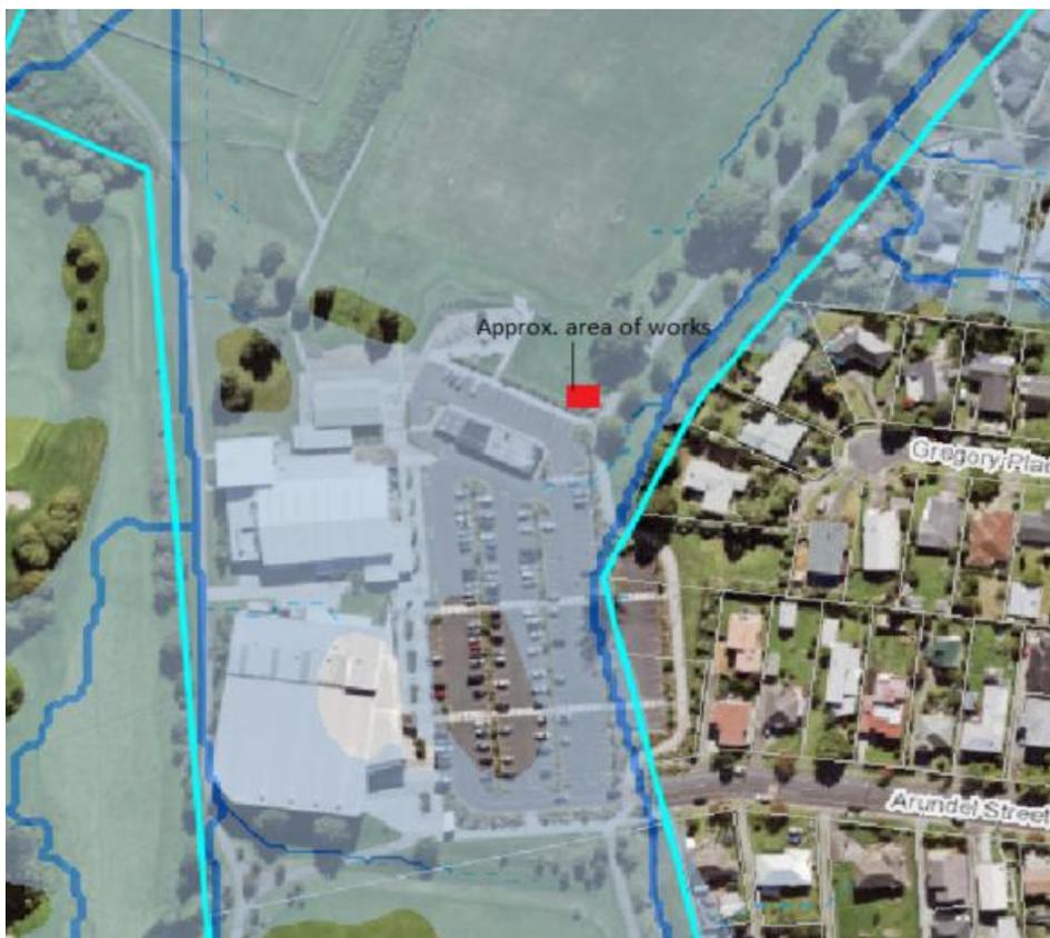
Figure 2.2: Proposed works in relation to floodplain (overlay in blue) and overland flow paths (blue line) (site boundary in light blue, approximate area of works outlined in red). (Source: Auckland Council GeoMaps, 2020).
