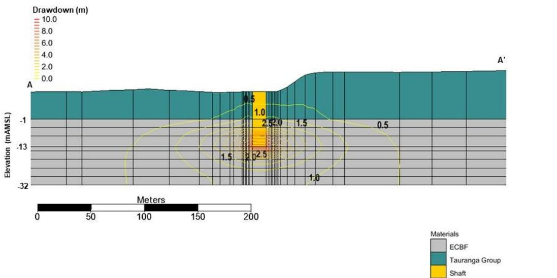
Figure 3. East-west cross-section of predicted drawdown under Scenario 6 conditions.
