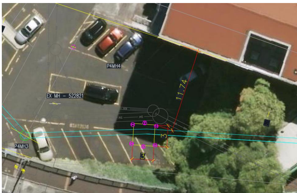
Figure 2-1: Site plan of the P3-P4 connector tunnel and shaft
