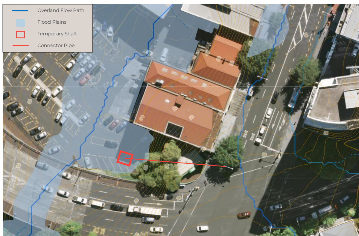
Figure 6-1: P3/P4 Connector and Greys Ave tunnelling shaft with stormwater features
