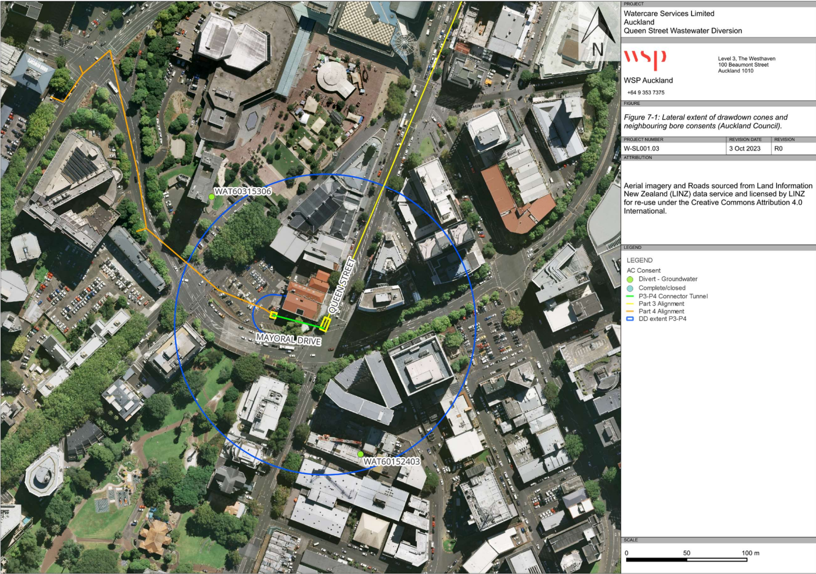
Figure 7-1: Lateral extent of drawdown cones and neighbouring bore consents (Auckland Council).
