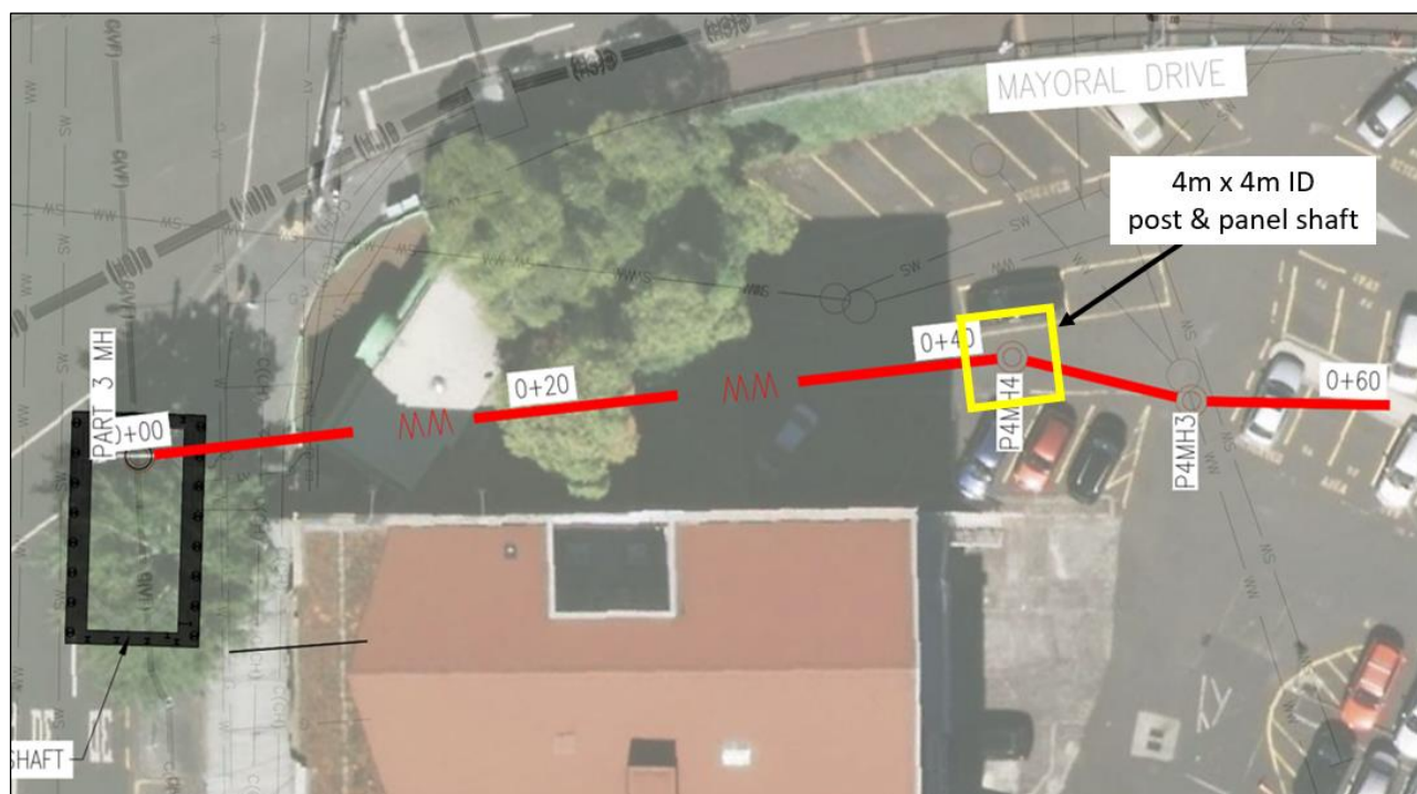
Figure 1.1: Site plan of the P3-P4 connector tunnel and shaft
