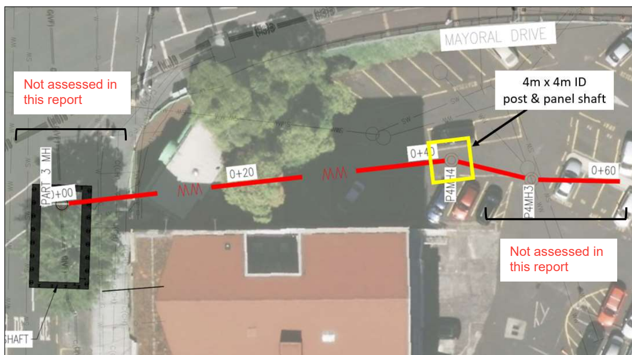
Figure 2-1: Site plan of the P3-P4 connector tunnel and shaft
