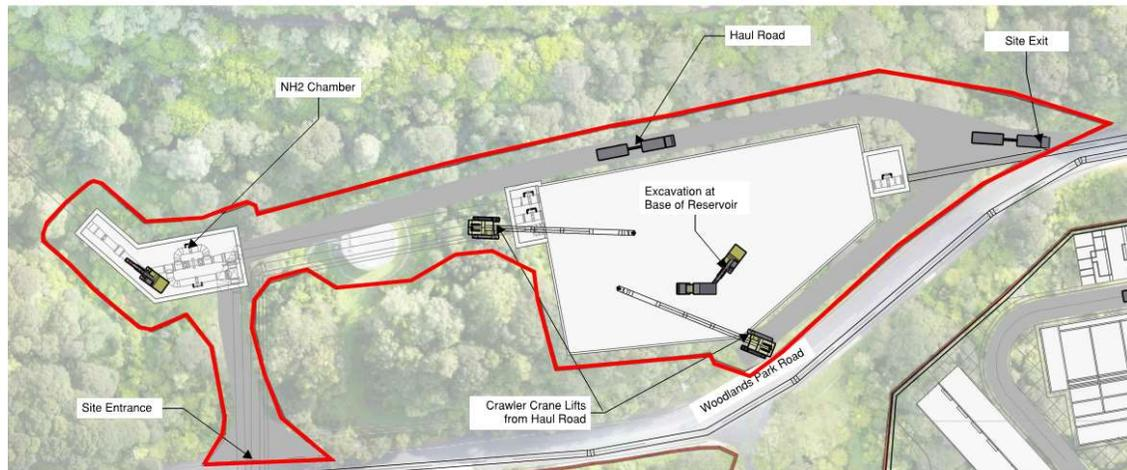
Figure 8 - Reservoir 1 Site Layout Plan
