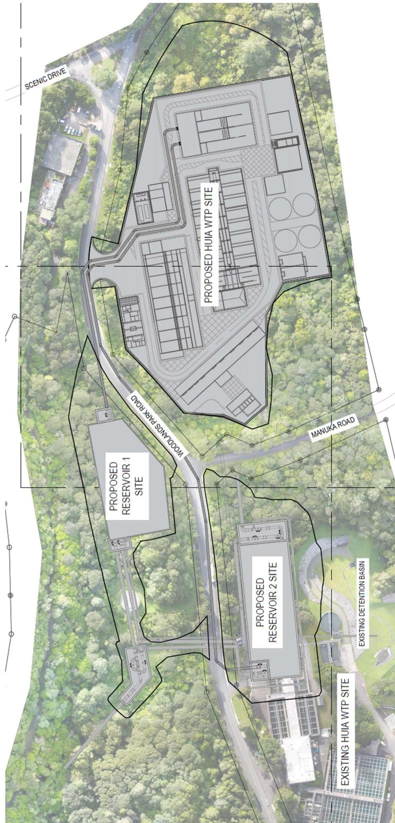
Figure 1 - General Arrangement of Proposed WTP and Reservoirs (Source: GHD dwg: 51-3357505-G001 [2])
