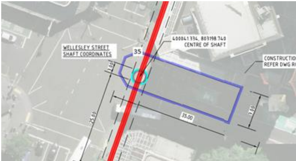
Figure 6 Wellesley Street Shaft position and compound
