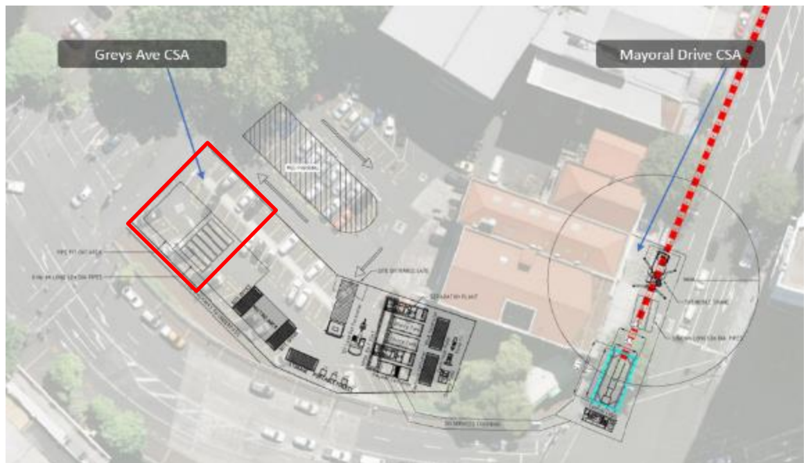
Figure 10. Greys Avenue CSA during tunnelling works, with red outline showing area where levelling earthworks will be required
