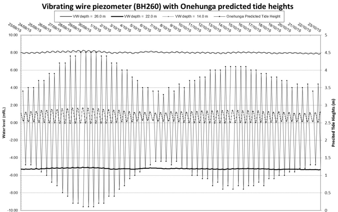
Figure 11.6 Vibrating wire piezometer results from BH260 for 30 days with predicted tide heights for Onehunga. Daily fluctuations in piezometer results appear comparable to predicted tide heights for Onehunga
