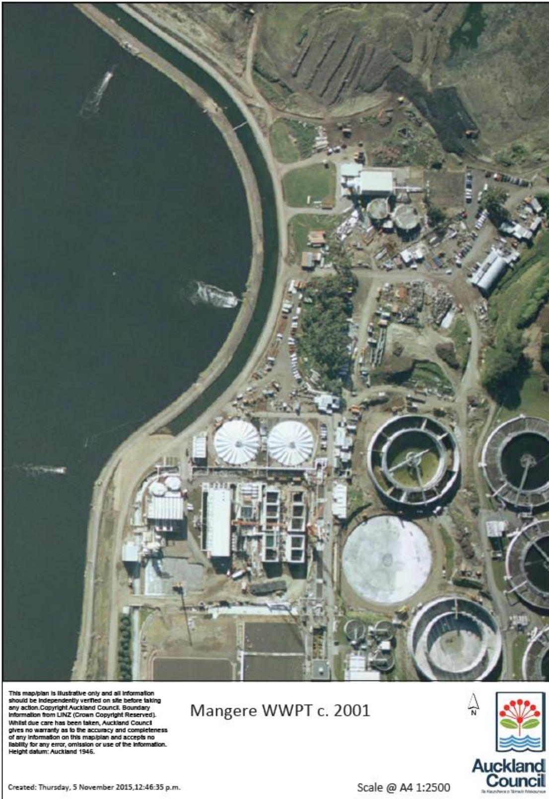
Figure 11.2 Aerial Photograph of Mangere WWTP circa 2001. Ponds appear to be being filled where the proposed emergency pressure relief chamber and rising mains will pass.
