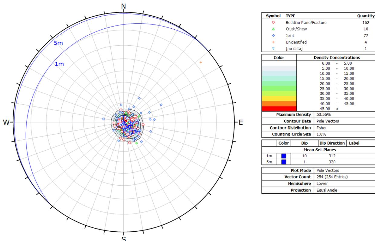
Figure 11.9 Stereonet of discontinuities for BH250. Discontinuities dip between 0° to 20°.
