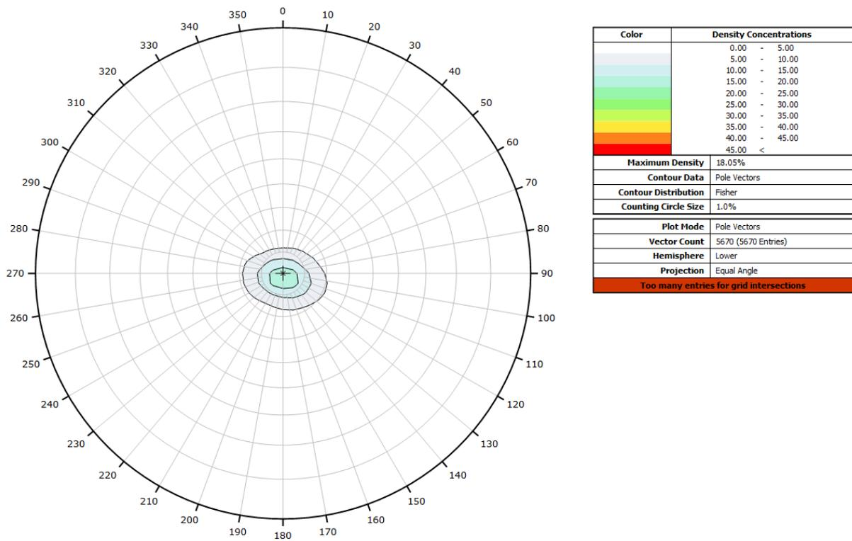
Figure 5.8 : Contour plot of all bedding planes and bedding fractures identified during televiewer logging.
