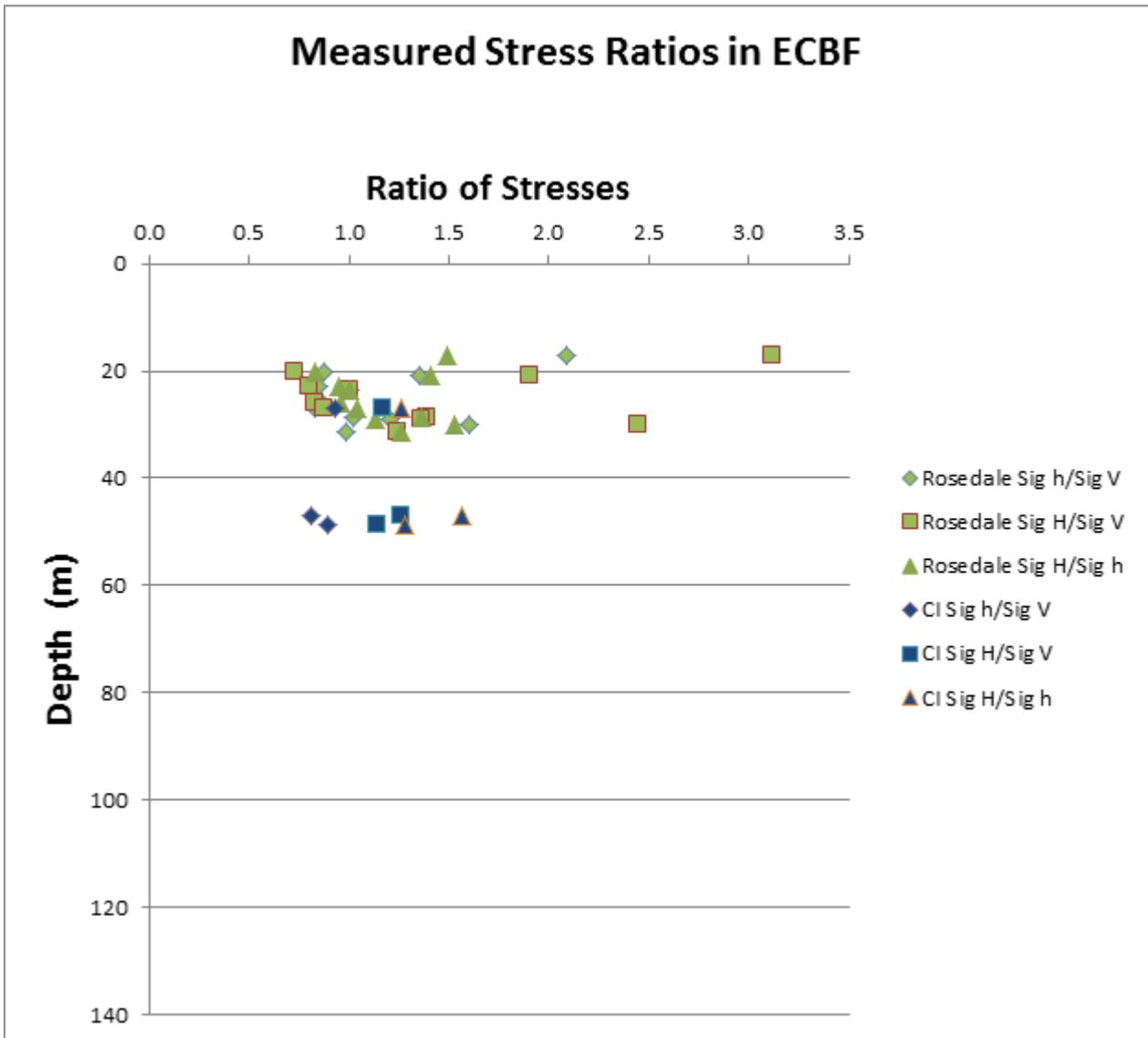
Figure 8.2: Measured Stress Ratios in ECBF (Hydraulic Fracture Method)
