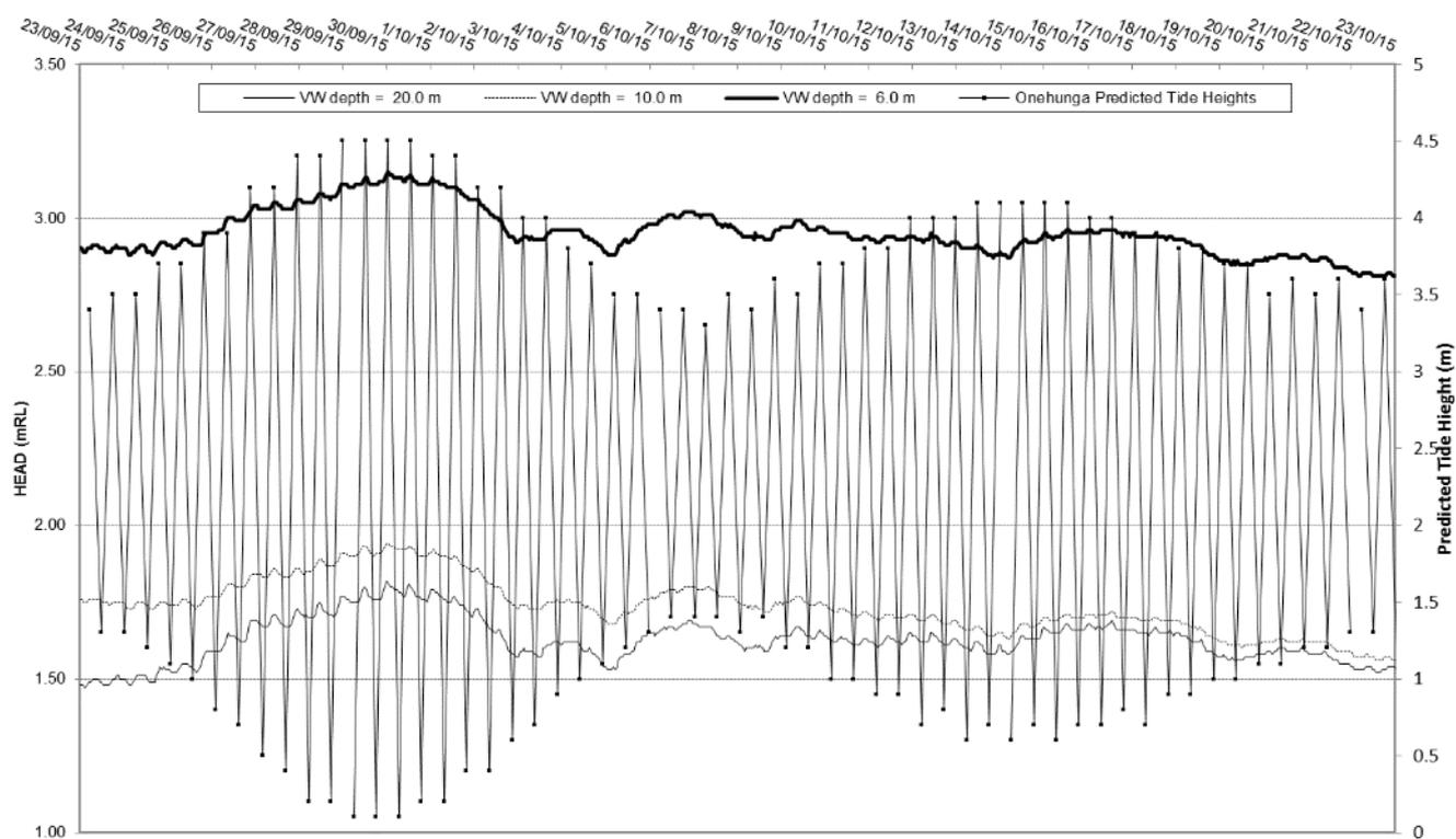
Figure 11.3 Vibrating wire piezometers in BH271 are compared with predicted tide heights for Onehunga. While fluctuations up to 100mm are observed it appears the overall groundwater trends are dominated by other factors.
