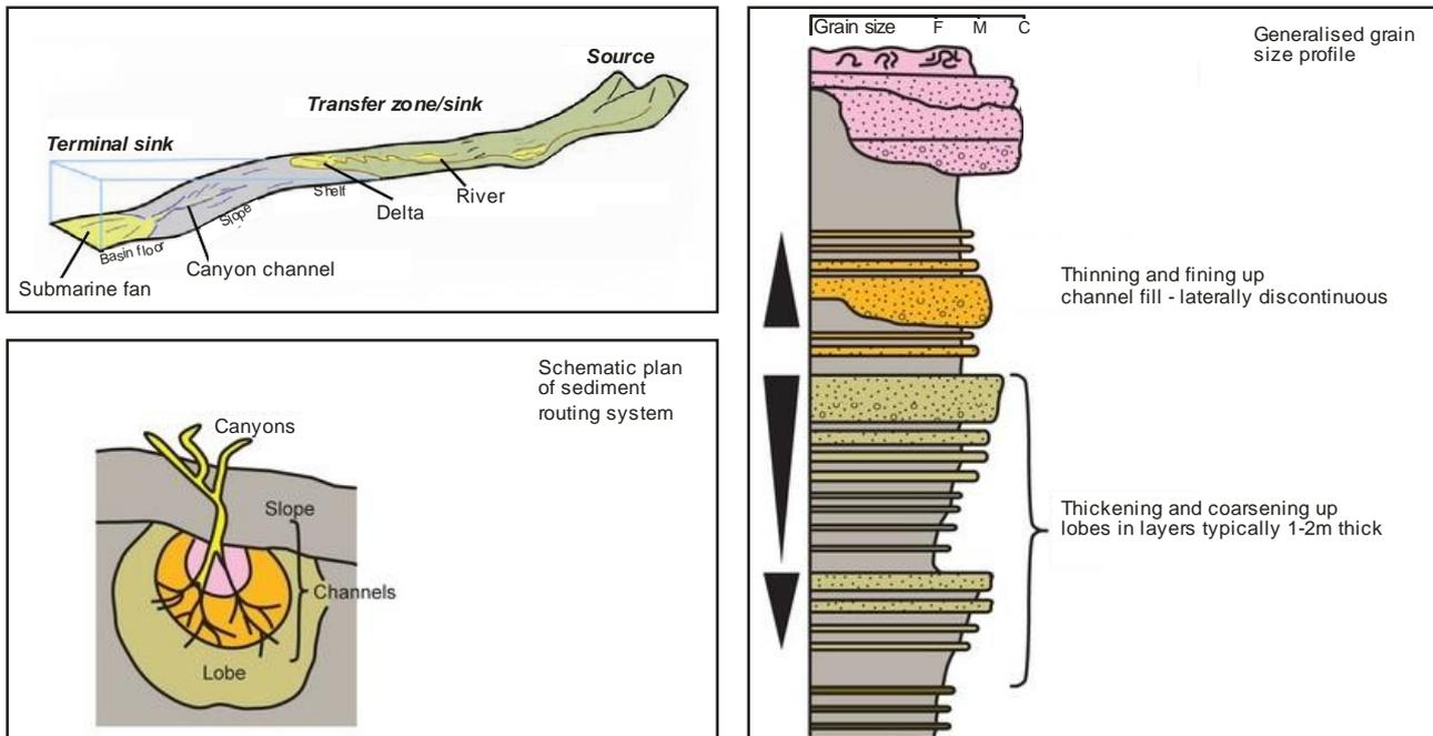
**Figure 3.1 : Overview of the depositional environment of the Waitemata Group showing the relationships between mudstone (grey), fine sandstone (green), course volcaniclastic sandstone (orange) and Parnell Volcaniclastic Conglomerate (pink).**
