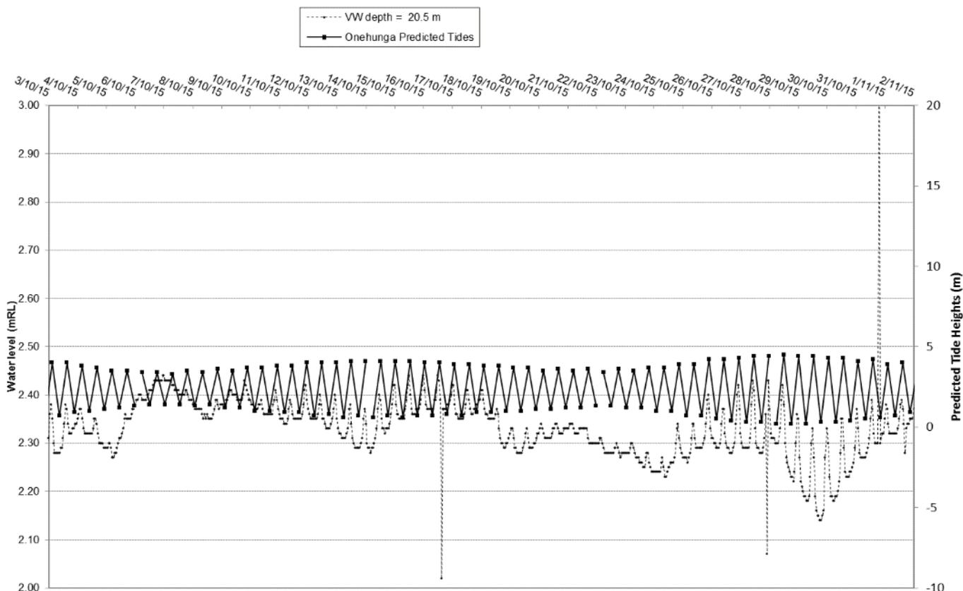
Figure 11.8 Vibrating wire piezometer results from BH255 for 30 days with predicted tide heights for Onehunga. Daily fluctuations in piezometer results appear comparable predicted tide heights for Onehunga. Notwithstanding, the tidal effects are very minor in relation
