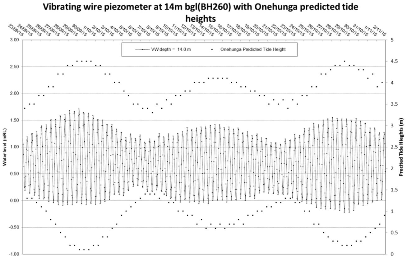
Figure 11.7 Results from vibrating wire piezometer installed at 14mbgl from BH260 for 30 days with predicted tide heights for Onehunga. 6 hourly fluctuations in piezometer results up to 1.7m are observed with spring tides showing greater variation than neap tides
