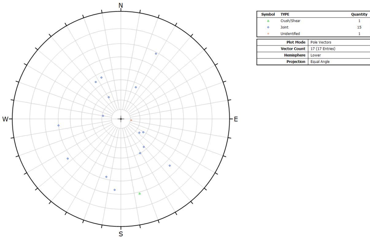
Figure 11.14 Stereonet of discontinuities in basalt for BH224
