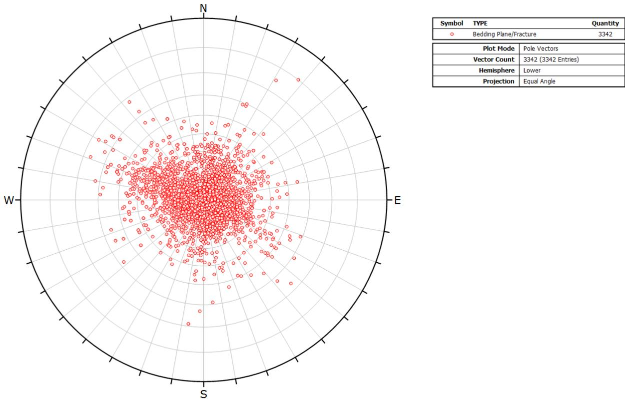
Figure 5.7 : Stereonet plot of all bedding planes and bedding fractures identified during televiewer logging.
