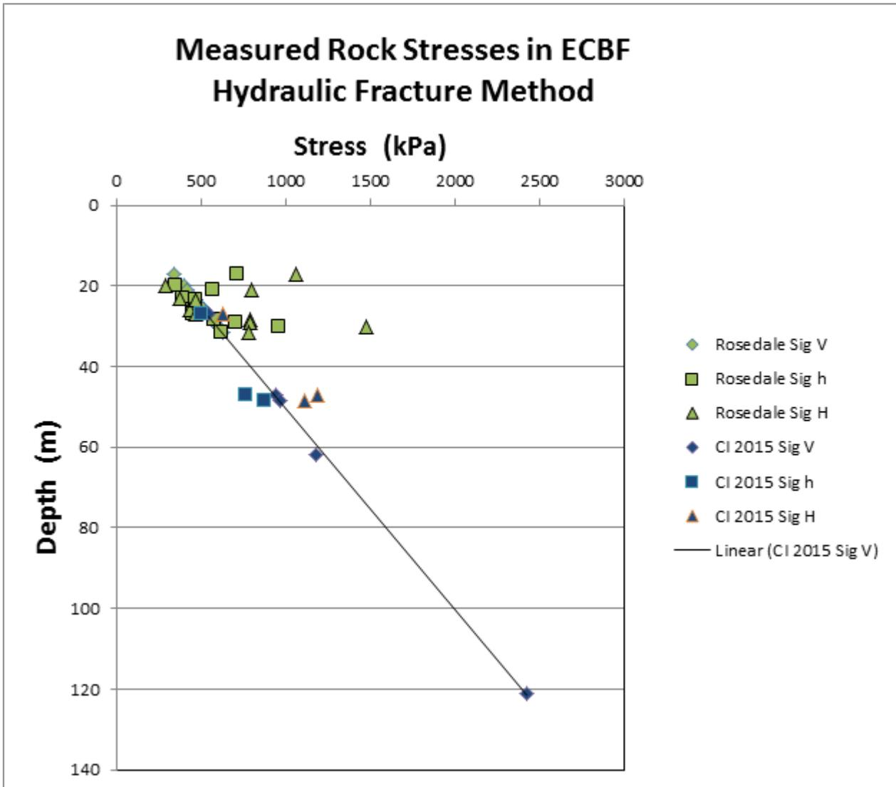
Figure 8.1: Measured Rock Stresses in ECBF (Hydraulic Fracture Method)
