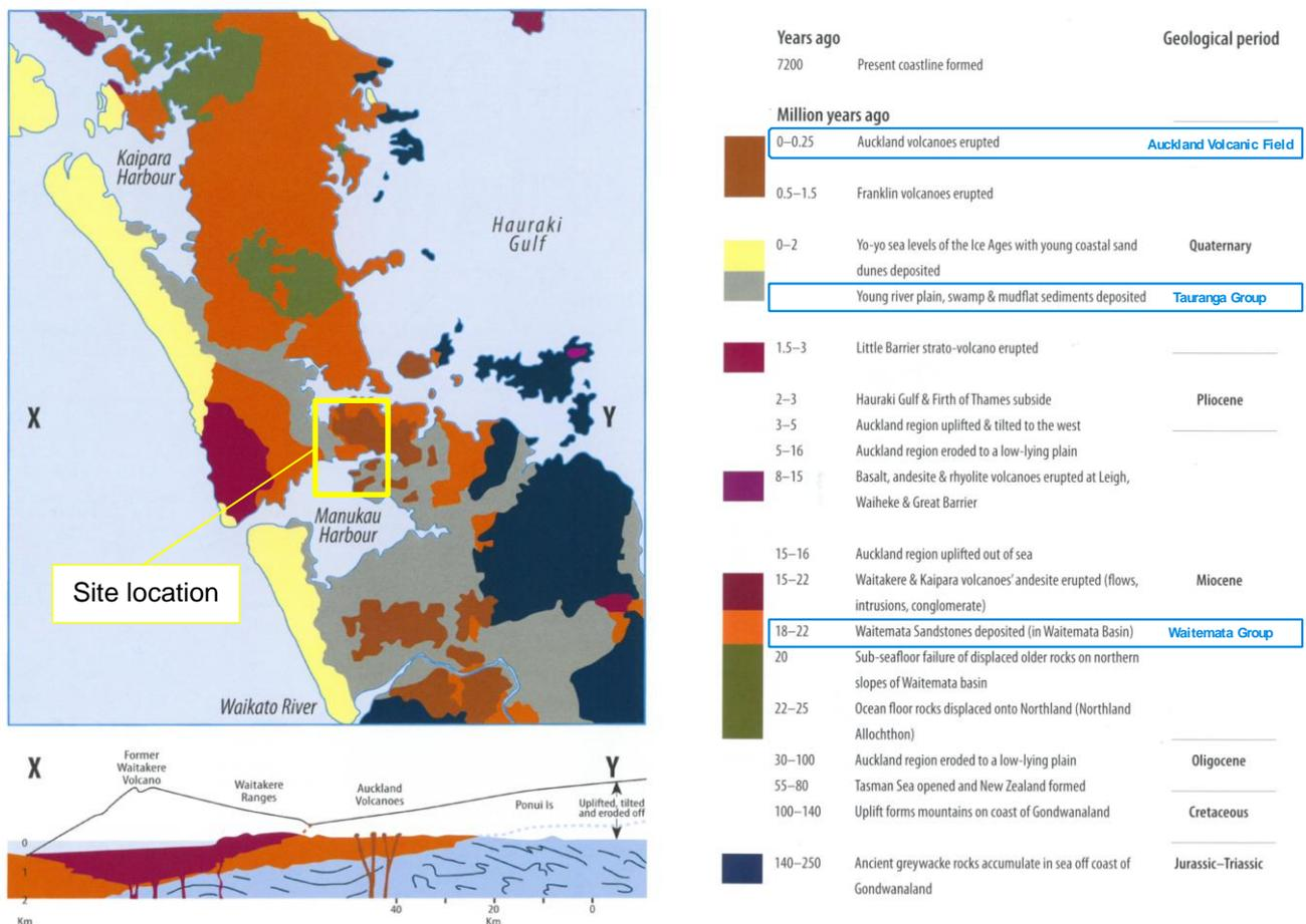
Figure 2.1 : Auckland simplified geology (Cameron, Hayward, & Murdoch, 2008) with the key geological units for the central interceptor project highlighted with blue boxes. Section shows the relative vertical positions of each unit.
