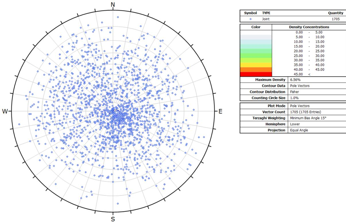
Figure 5.11: Stereonet plot of all joints recorded during televiewer logging (no contours shown as density too low)
