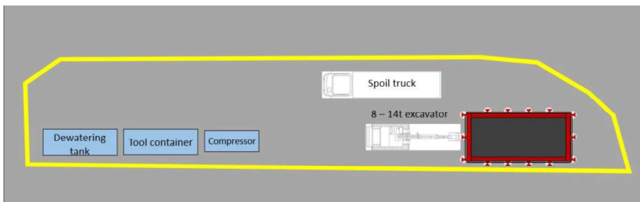
Figure 3 Mayoral Drive CSA layout during shaft construction
