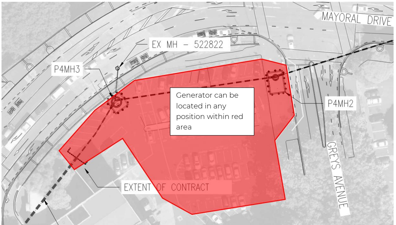
Figure 5-2: Location of dewatering generator at Greys Ave CSA
