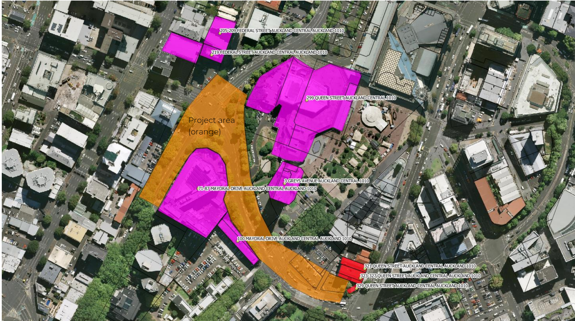
Figure 6-1: NSRs which are predicted to exceed the noise criteria from works within the road zone (pink) and outside of the road zone (red) at any stage/phase
