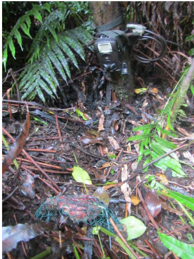
Figure 2: Camera trap set-up with the lure (comprising 150 g fresh rabbit meat between two pieces of Connovation's Erayz wrapped in chicken wire) pegged to the ground c.60cm in front of the device. Image from DOC's interim camera trapping guidelines (Gillies, 2021).
