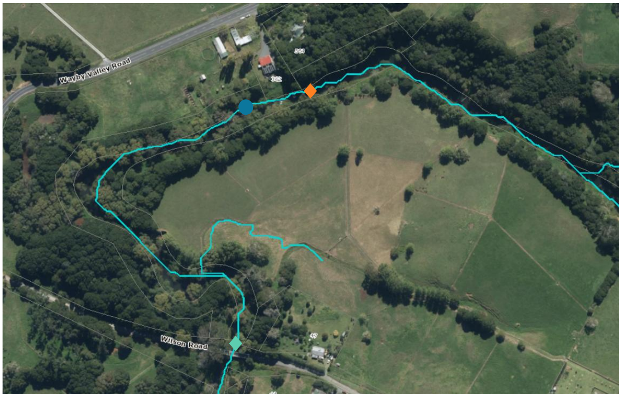
Figure 1-1 Aerial image of Wellsford water treatment plant alongside the Hōteō River showing the intake sample point (orange diamond), discharge sample point (circle) and downstream sample point (green diamond).
