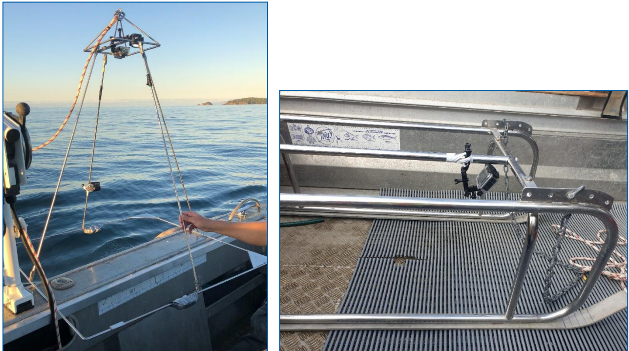
Figure 12. Left: Drop camera frame with the dual camera system in position to drop to the seafloor. Right: sled used for the video transects in surveys prior to 2023.
