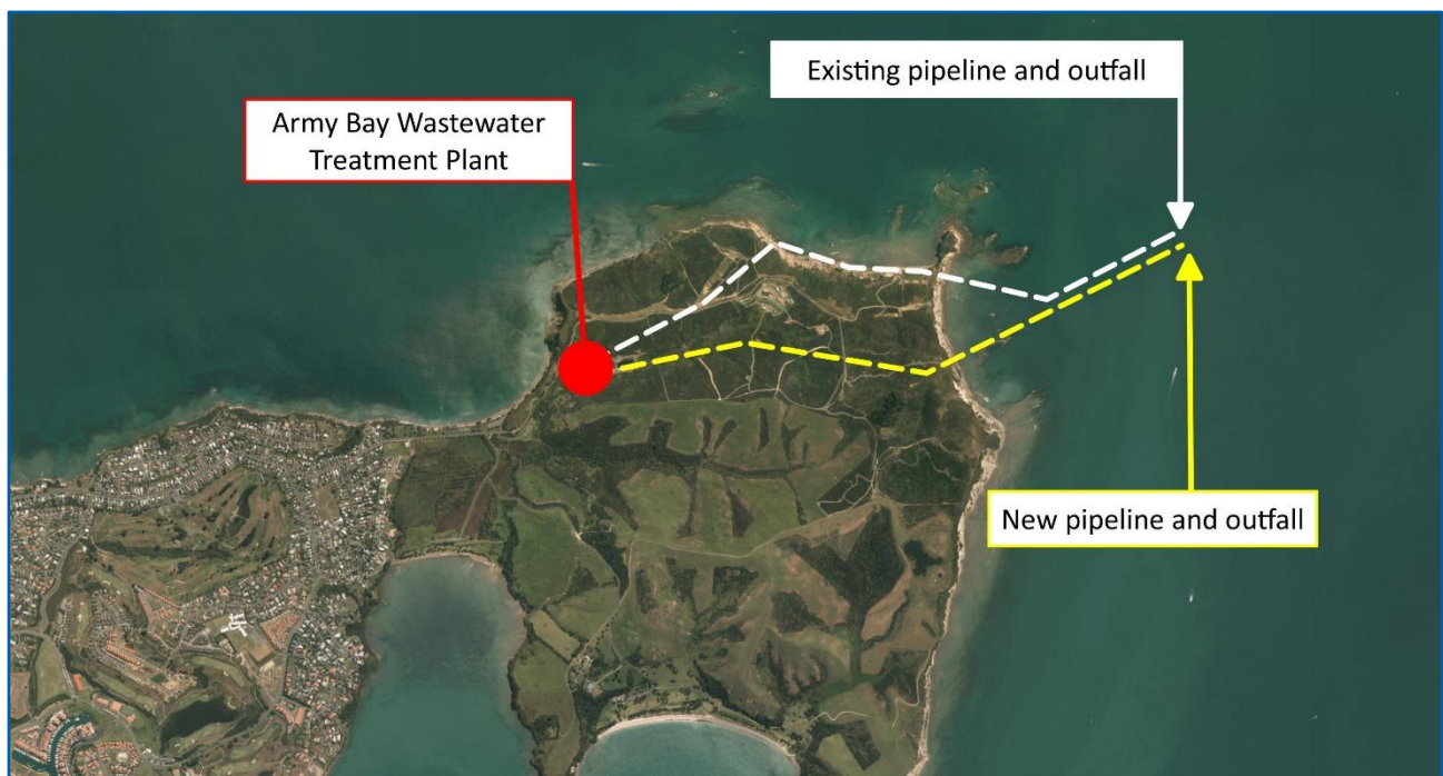
Figure 1. Map representing the route of the old (labelled existing) and new pipeline and outfall. From Watercare Services.
