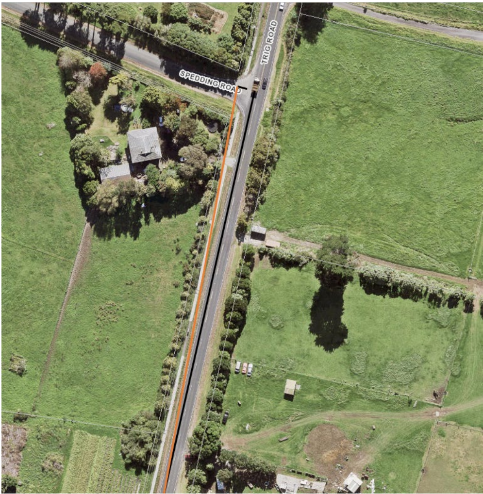
Figure 2: Sight distance south at the Trig Rd / Spedding Rd intersection (sight distance calculation lines in black, vegetation clearance extent between black and orange lines)
