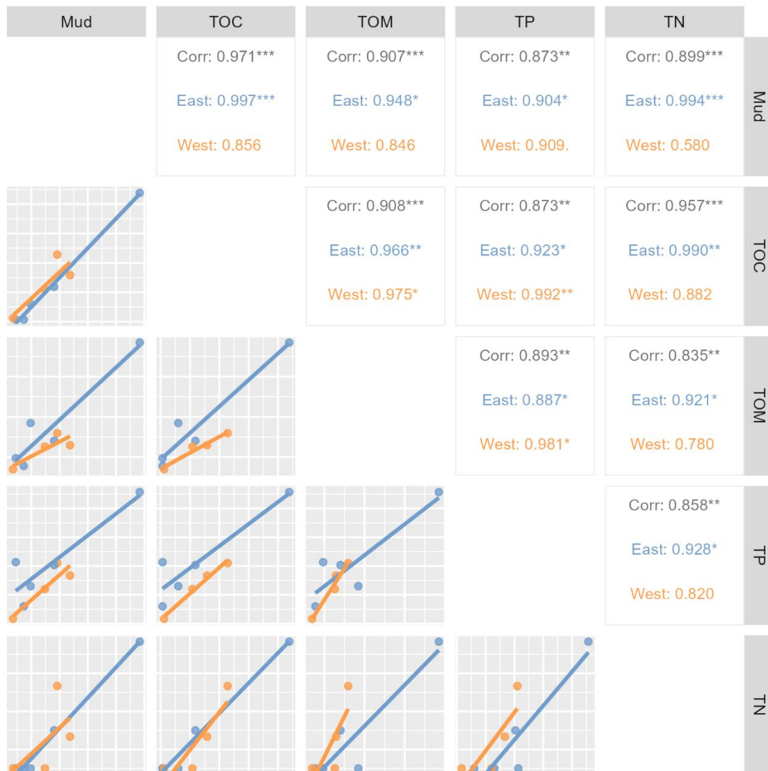
Figure 28: Correlation matrix showing the strength of relationships between percent mud (Mud), total organic carbon (TOC), total phosphorus (TP) and total nitrogen (TN) concentrations. Correlations are provided for pooled data and for sites on the eastern and western sides of the channel.
