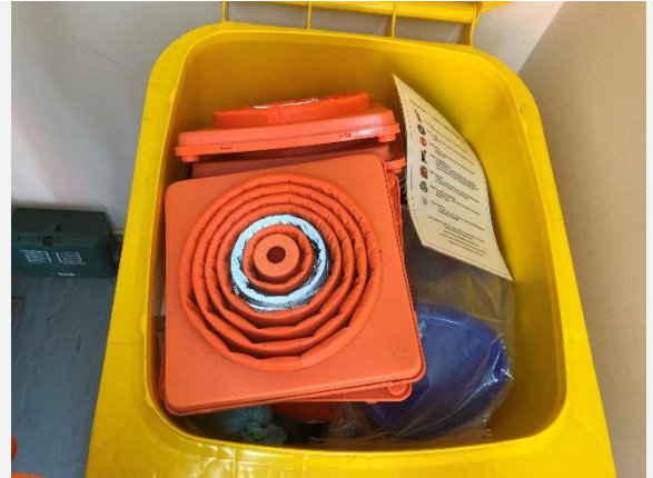
B: Emergency spill kit in control room
