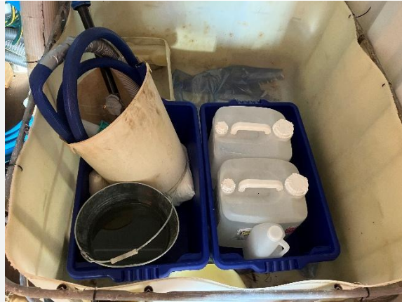
A: Portable chemical bund in workshop container
